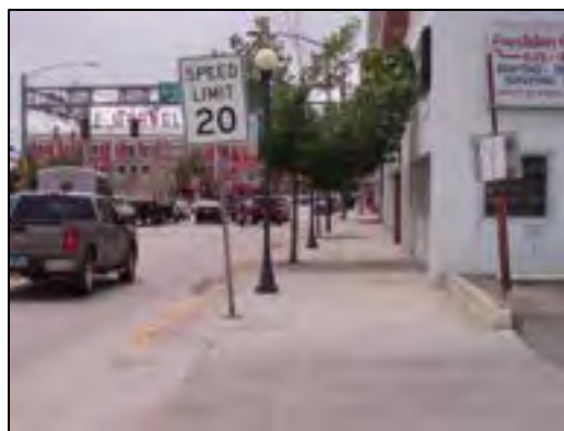
Figure 62. Human scale lighting helps delineate pedestrian friendly environments by illuminating the sidewalk.
