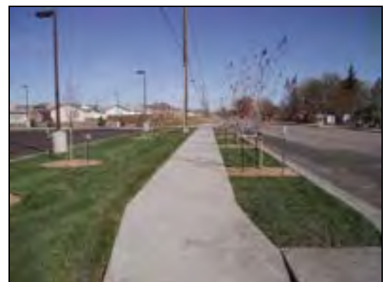
Figure 53. Physical separation from the roadway increases the comfort of the pedestrian environment
