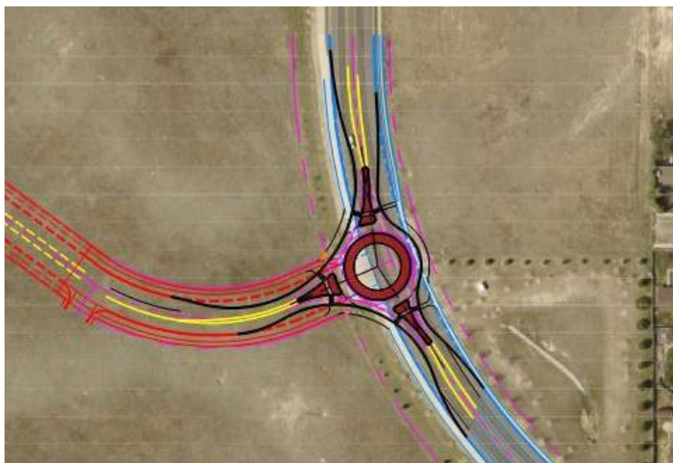
Figure 8: 3-Leg Roundabout Design for a Future Carlson Street Intersection with Converse Avenue
