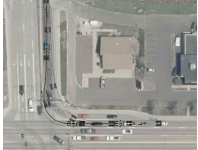
WB-53 Semi Truck with Pup Turning Requirement
