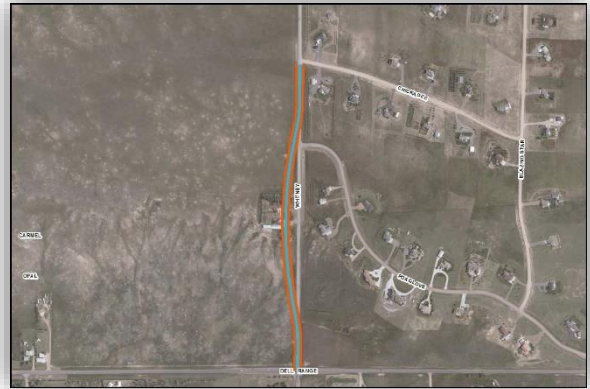
Figure 5.8 Alternative 5: Three-lane Roadway, Revised Alignment, Accessible Profile, and Impact to Plains All American Pipeline (PAAPL)
