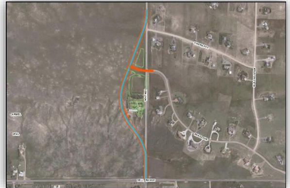
Figure 5.9 Alternative 6: Three-lane Roadway, Revised Alignment, Accessible Profile, No Impact to Plains All American Pipeline (PAAPL) or Whitney Gysel Barn Structure
