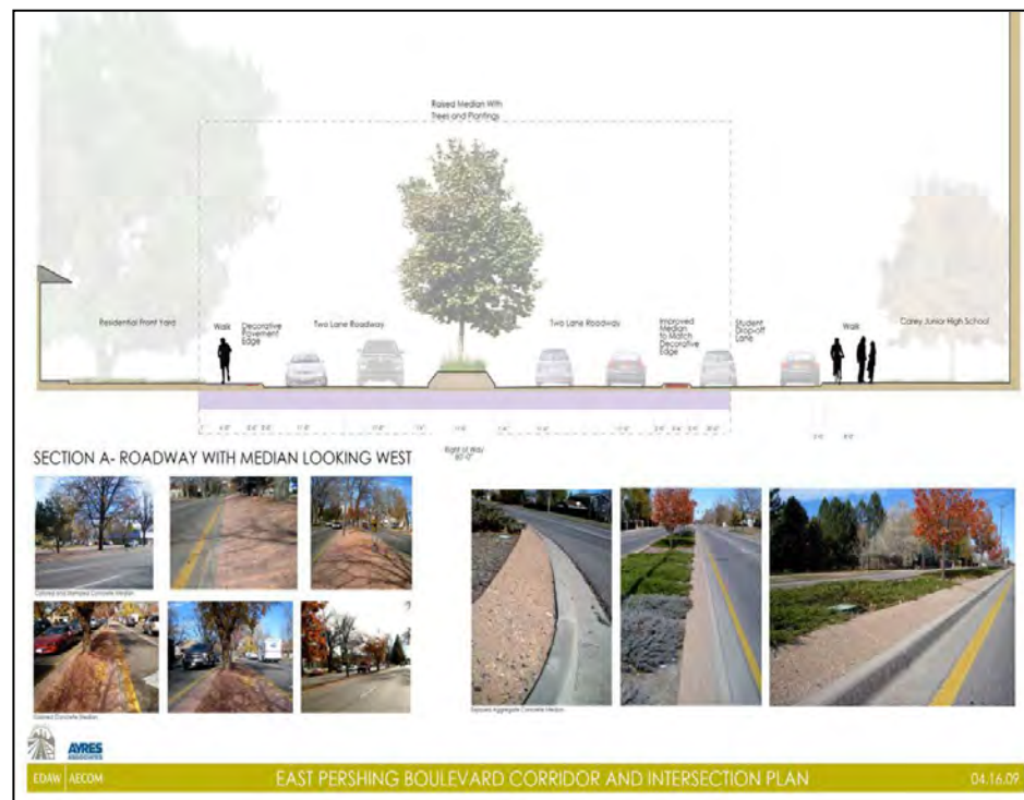
Proposed East Pershing Blvd. Median using Monolithic Concrete Coloring Additive with Exposed Aggregate Texturing and Coloring Option D
