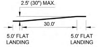
c. Ramps vs. Import Fill – After the bridge has spanned the railroad ROW we have to bring the pathway back down to grade. Some of the greenway options require a ramp as existing ground is much lower than the bridge structure. A ramp can be constructed from steel, as shown in the photo below, or it can be constructed by building up fill material to the elevation necessary. A steel structure can be prefabricated to look like the bridge itself.
