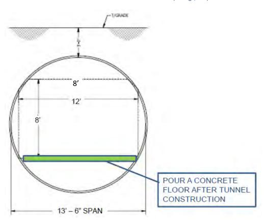
Pipe as a Tunnel: Multiplate Arch / Corrugated Steel
