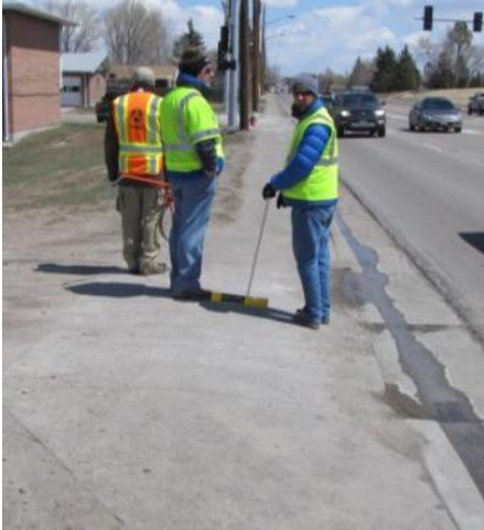
Exhibit 87 Looking East at Driveway Cross-Slope at Greybull Avenue
