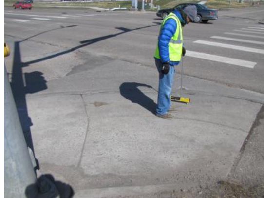
Exhibit 36 Slope of Pedestrian Ramp in SW Corner
