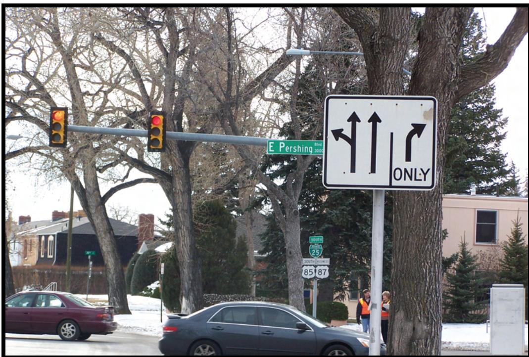
**Figure 80 Lane Control Sign for Southbound Approach on Central**
