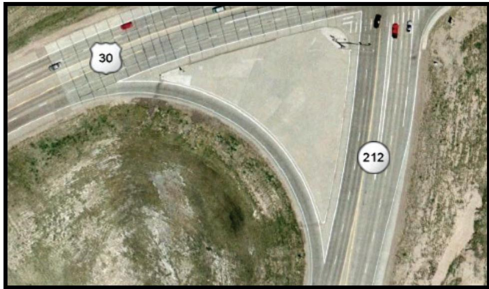
**Figure 26 Channelized Right Turn from EB E Lincolnway to SB College**
