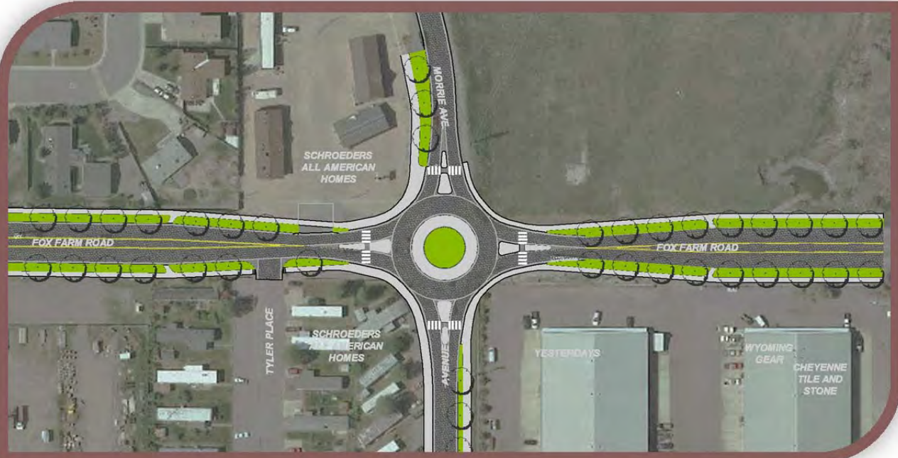
Proposed Intersection Improvements at Fox Farm Rd and Avenue C / Morrie Avenue – Roundabout
