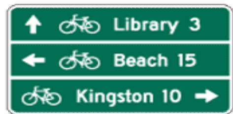
Figure 4. MUTCD sign D1-3C can be used for wayfinding with or without distance information.
