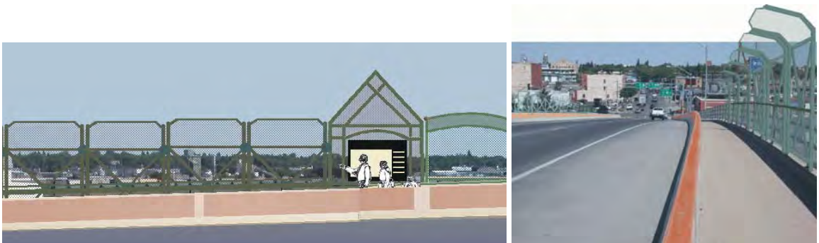
Figure 5. Bridge Rail Alternative C
