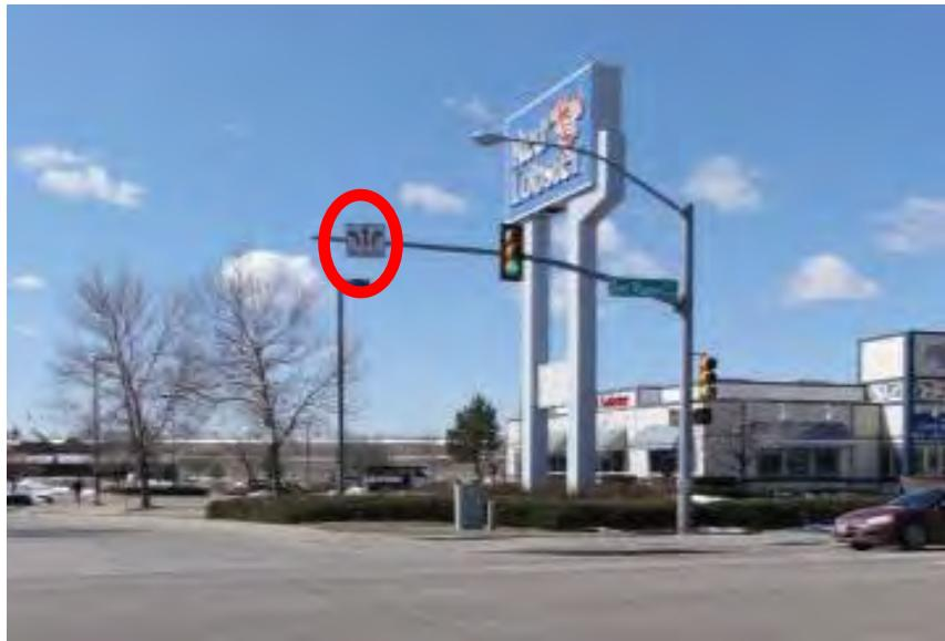
**Exhibit 56 Low Reflectivity of Channelization Sign Mounted to Mast Arm Signal Pole****Description of Safety Issue:**
