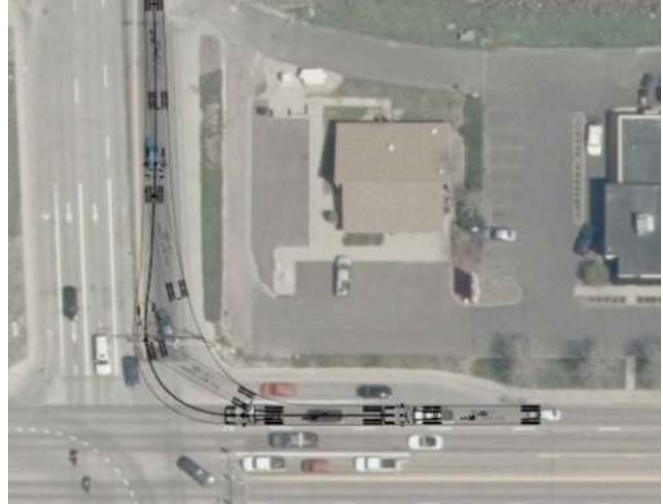
WB-53 Semi Truck with Pup Turning Requirement
