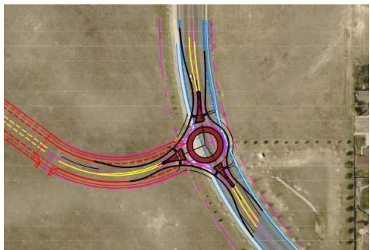
Figure 8: 3-Leg Roundabout Design for a Future Carlson Street Intersection with Converse Avenue
