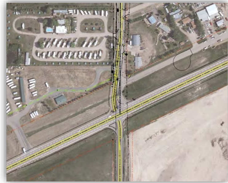
Figure 5.14 Realign Intersection/ Remove Skew
