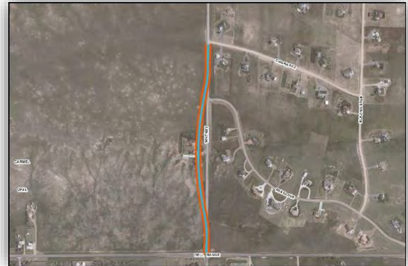
Figure 5.8 Alternative 5: Three-lane Roadway, Revised Alignment, Accessible Profile, and Impact to Plains All American Pipeline (PAAPL)
