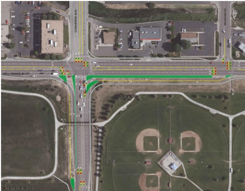
Figure 3-10 - CFI Modified Concept
