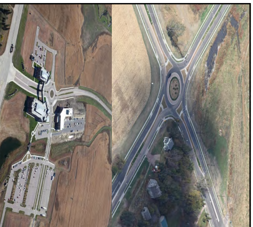
Modern roundabouts maximize intersection capacity and enhance safety, particularly for intersections with high left-turn volumes
