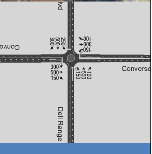
Modern roundabouts maximize intersection capacity and enhance safety, particularly for intersections with high left-turn volumes
