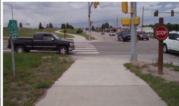
Installation of stop lines can provide visual guidance for motor vehicles on where to stop and help keep crosswalks clear for bicyclists and pedestrians.
