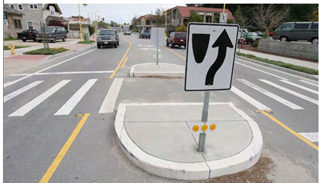
Figure 19. Pedestrian refuge islands reduce pedestrian exposure at roadway crossings.
