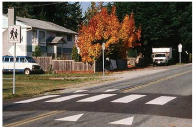
Figure 33. Raised crosswalks increase pedestrian visibility. Source: www.walkinginfo.org
