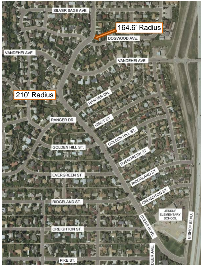
Figure 2 - Evers Boulevard Centerline Curve Radii
