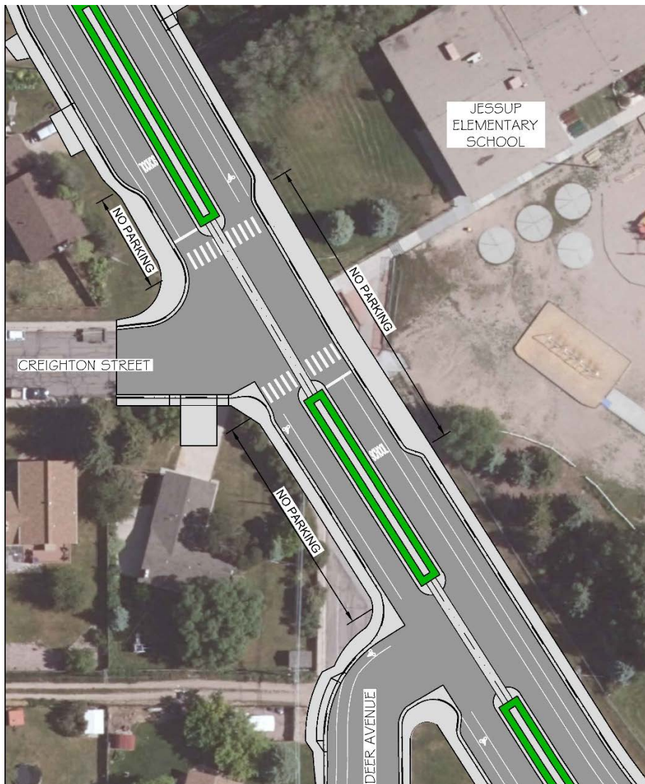
Figure 3 - Jessup Elementary Additional Crosswalks and Curb Extensions
